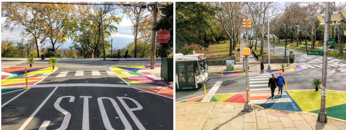
Images. Temporary curb extensions in Jersey City help in enhancing pedestrian safety. It also provides an opportunity to create a unique park identity by means of cost-efficient tactical urbanism solutions. Photos taken by Streetplans.
