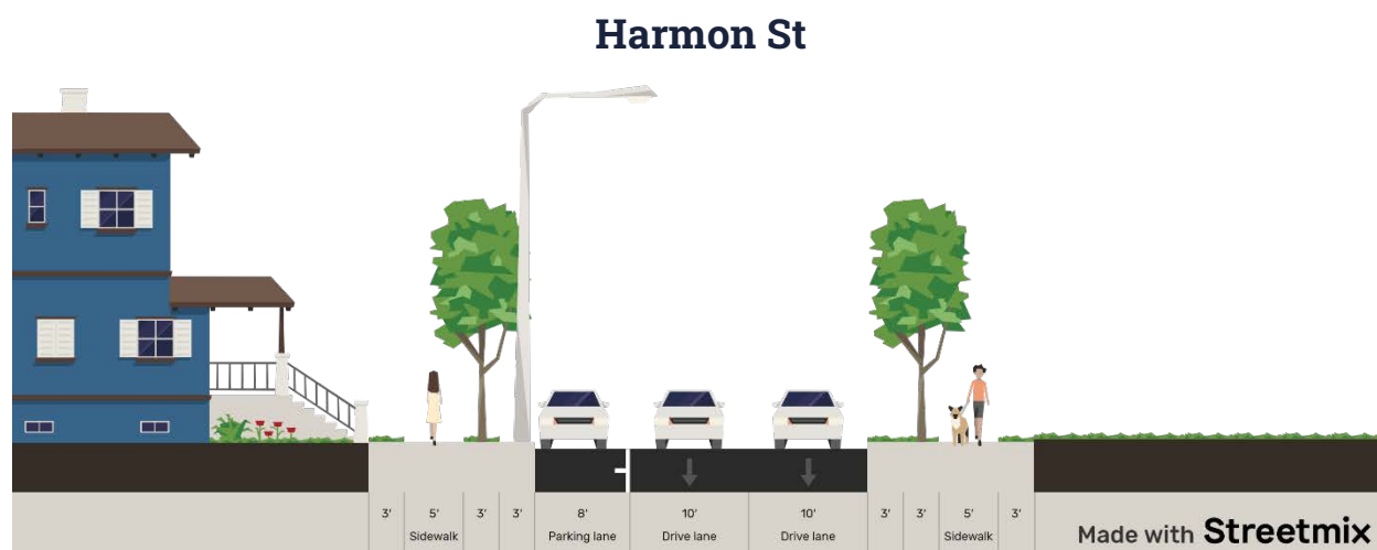
Figure 19. Street cross-section of Harmon Street. The park is to the right of the street which has two drive lanes, sidewalks on both sides, and a parking lane on the left, next to the neighborhood residences. Diagram created in Streetmix by EC, 2022.
