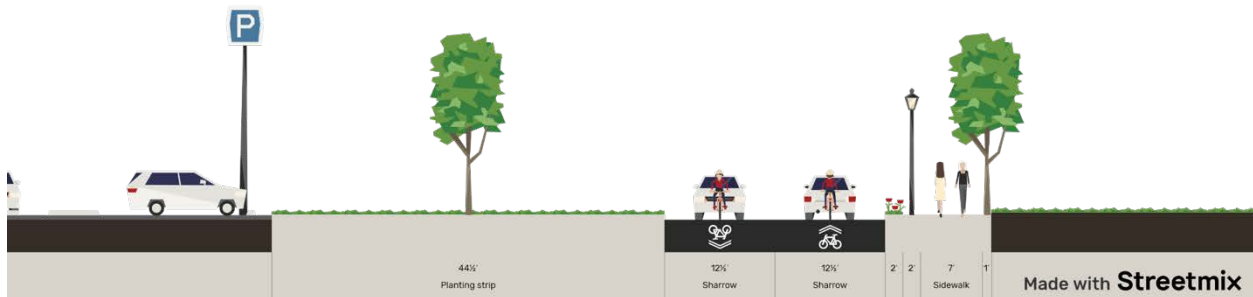
Figure 64. Proposed layout for Collat Avenue looking north from the community center. The new design includes an ADA-compliant pathway set back from the road, pedestrian-scale lighting, and bike sharrows on the road. Diagram created in Streetmix by EC, 2022.
