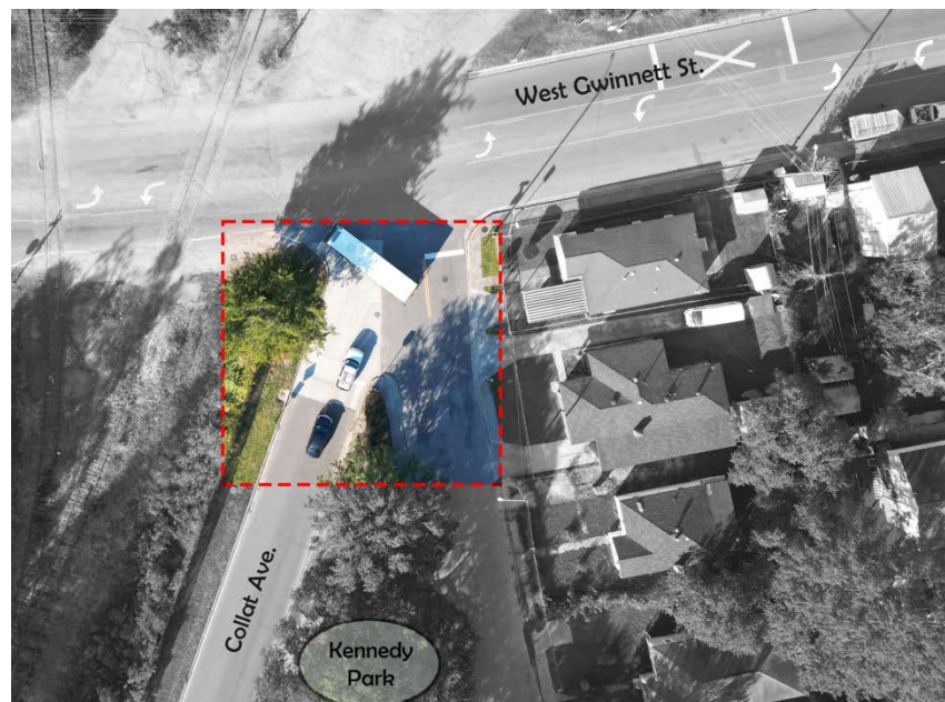
Image. The cross-traffic pattern created by the combined West Gwinnett Street/Collat Avenue/Carroll Street intersection. The first of the two cars in this image have advanced beyond the Collat Avenue stop sign but then had to yield to the CATS bus turning onto Carroll Street. Photo taken by EC, 2022.
